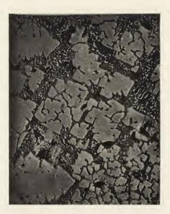
Fig. 9. Crystals of Al<sub>2</sub>Cu. Magnified 150 diameters.
